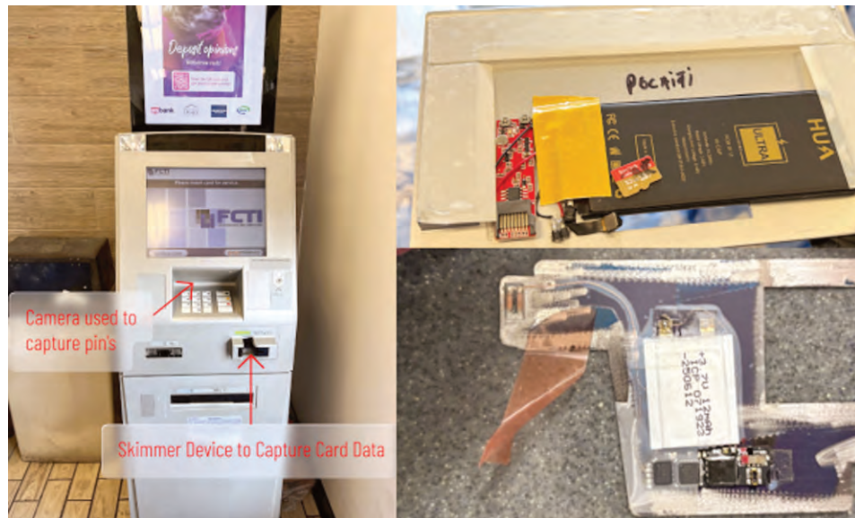
Photos of skimming devices recovered
